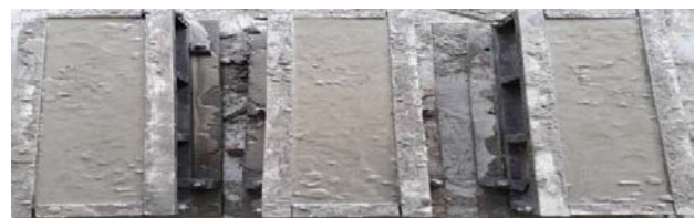
Figure 3 Casting of samples
