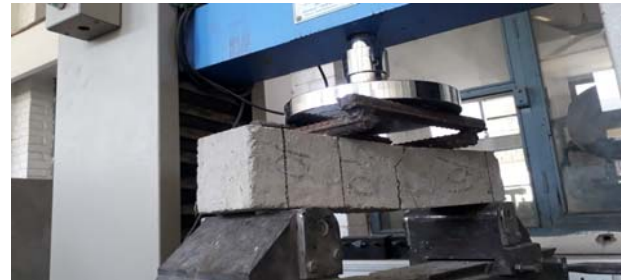
Figure 29 Beam failure (flexure)
