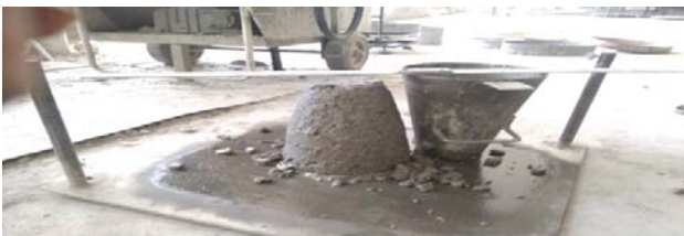
Figure 5 Slump test of concrete
