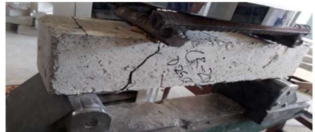
Figure 30 Beam failure (shear)
