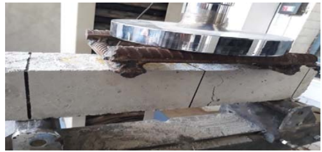
Figure 28 Beam failure (flexure)
